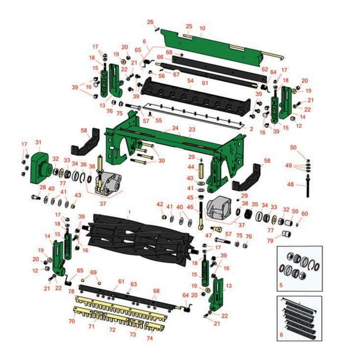
Cutting Unit - Serial up to 020000 Reel & Bedknife
