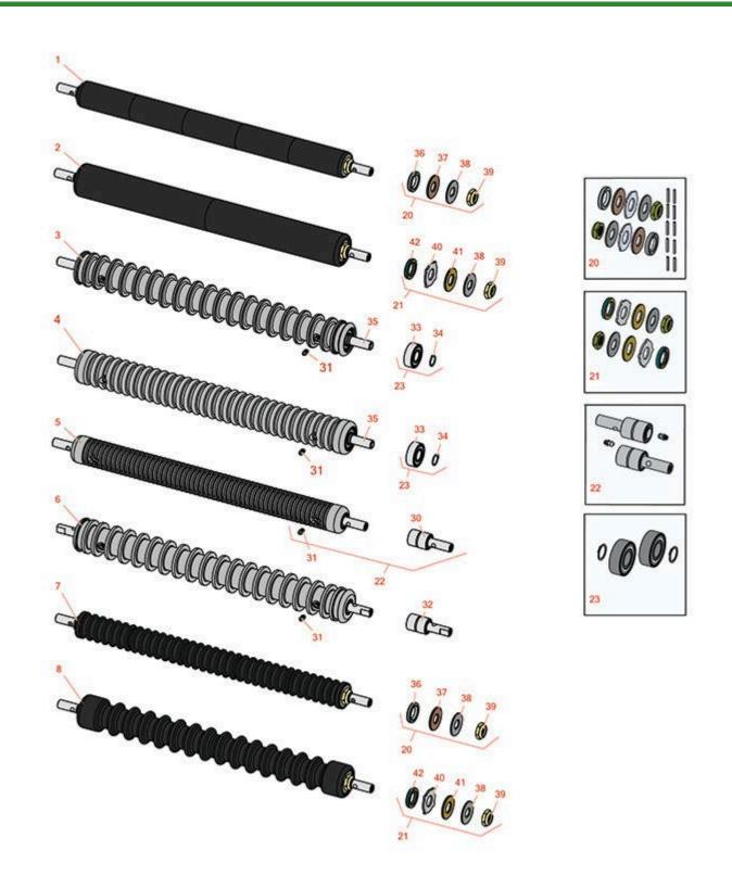
4-Bolt Cutting Unit - Models 04480 & 04481 Front Rollers
